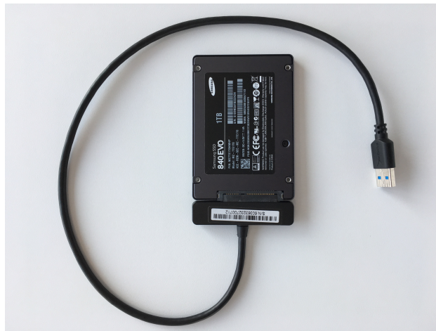
Figure5.5.: SATA-to-USB adapter with SSD attached.
