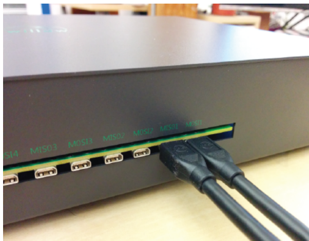
Figure4.2.: Example of Datanode paired-ports MISO1 and MOSI1 (left) connected to a headstage's MISO/MOSI ports (right).
