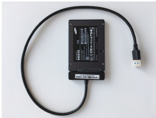
Figure3.3.: SATA-to-USB adapter with SSD attached.
