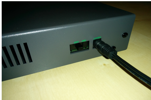
Figure3.1.: Datanode 12VDC power port and on/off switch.
