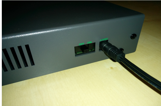
Figure4.1.: Datanode 12VDC power port and on/off switch.
